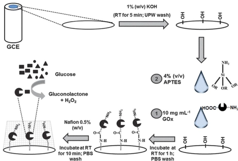
**Figure 5:** Bioanalytical procedure for the development of a highly-simplified mediatorless electrochemical glucose biosensor. Reproduced with permission from the Royal Society of Chemistry [19].
