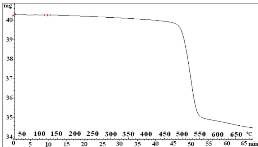
**Figure 3:** Thermal gravimetric analysis (TGA) of 100-230 mesh particles of diaspore.
