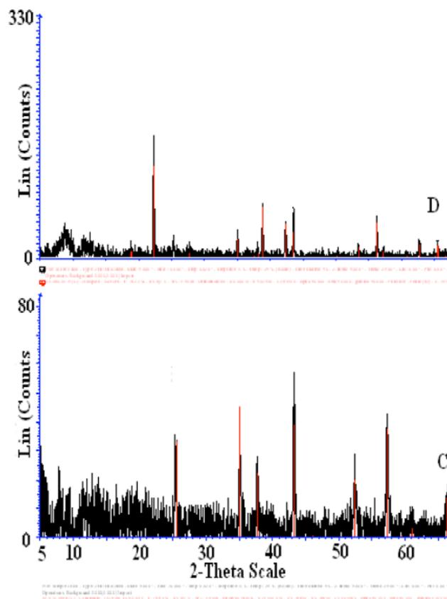
**Figure 2:** X-ray diffraction patterns of raw diaspore (D) and after heating for 1 hour at 600°C (C).
