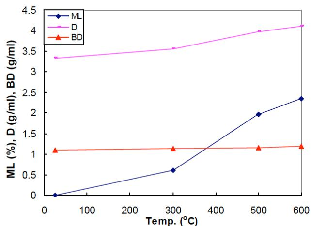
**Figure 1:** Variation in mass loss (ML), density (D) and bulk density (BD) with respect to temperature.
