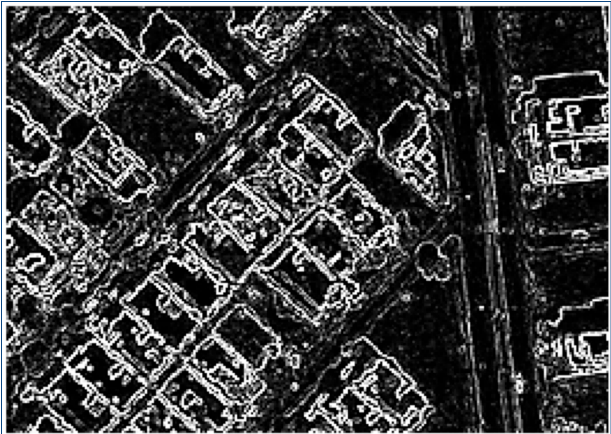
Figure 4: The implementation of edge extraction algorithm on sample satellite imagery to compute edge features. Note that edges of impervious surfaces such as residential building rooftops, roads, sideways, open spaces etc. have been extracted.
