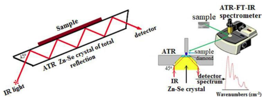
**Figure 1:** Schematic presentation of attenuated total reflection (ATR)- Fourier Transform Infrared technique. The Infrared light passes through a zinc-selenide (Zn-Se) crystal and after multiplication of the reflections (insert) the beam is collected by a detector
