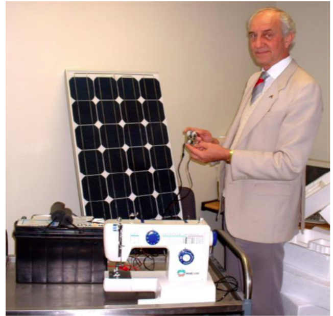
Figure 1: Author displaying the essentials of the 12v DC, battery-less, PV solar sewing machine.
