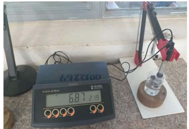
Figure 2: Benchtop HI2210 pH meter.
