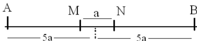
**Figure 4:** Sketch diagram of the Schlumberger array. (a: distance between the potential electrodes).
