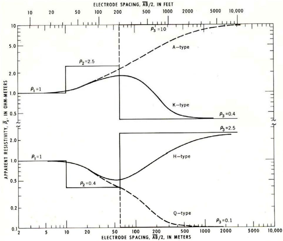
Figure 6: Examples of four types of the three layer Schlumberger sounding curves [21].
