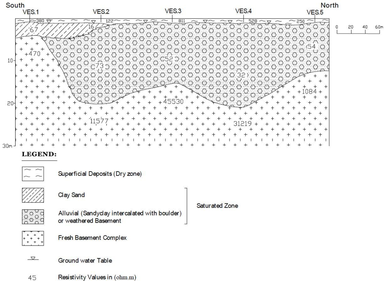
Figure 8: Geoelectrical Section for Duma Site.
