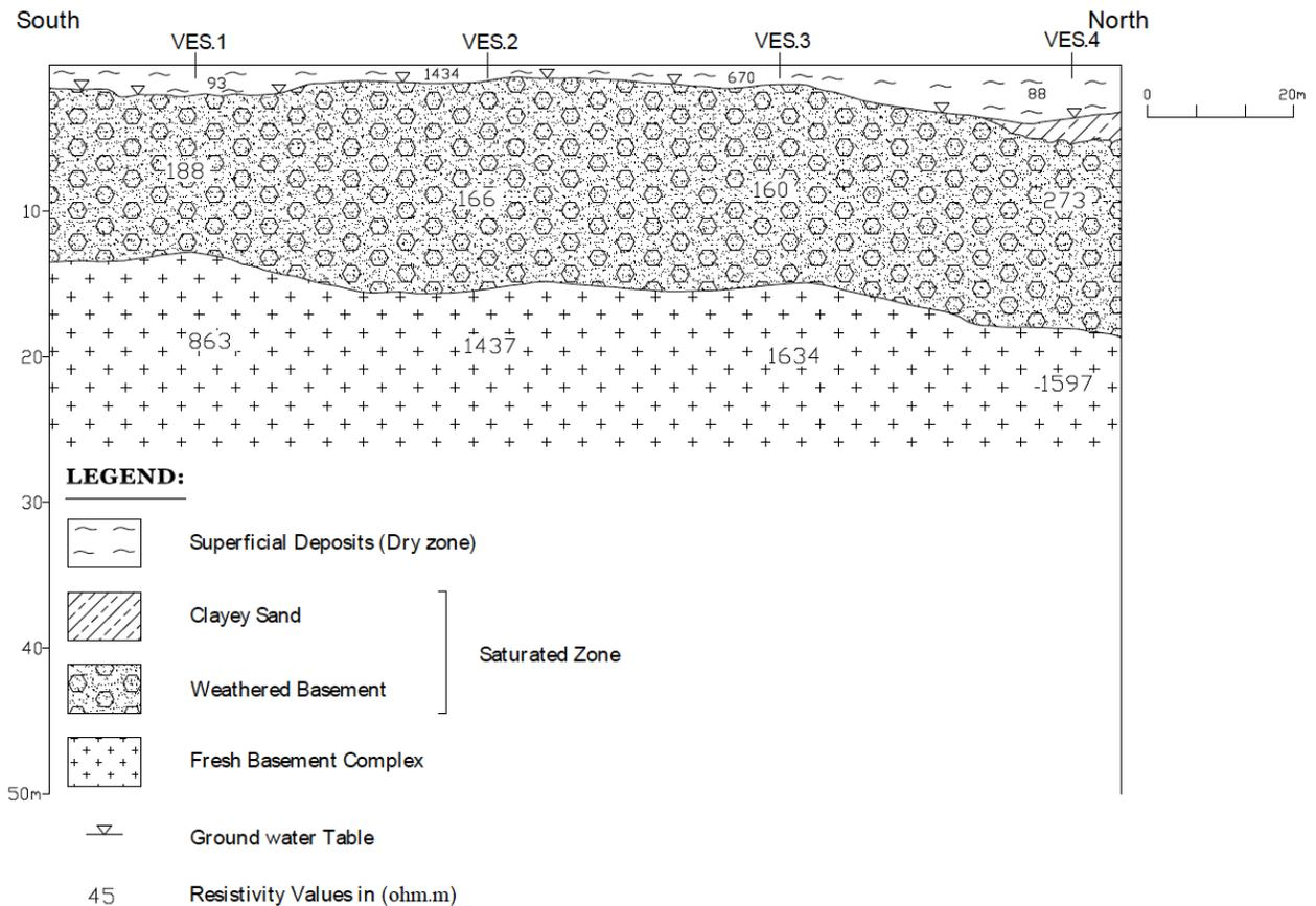
Figure 7: Geoelectrical Section for Andro Site.
