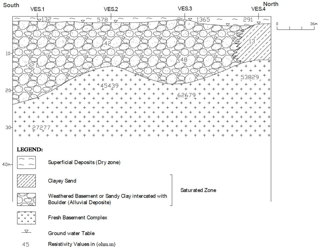
**Figure 9:** Geoelectrical Section for Manwashi Site.
