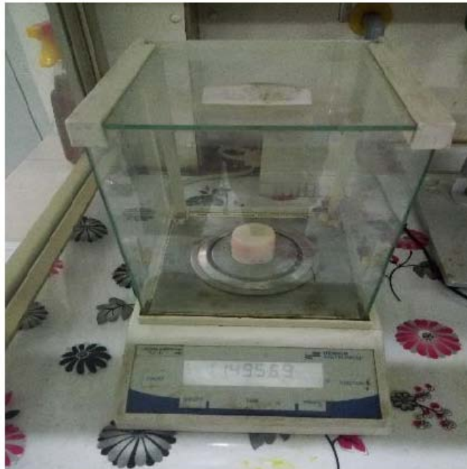
Figure S11: Balance electronic accuracy of 0.01 g.
