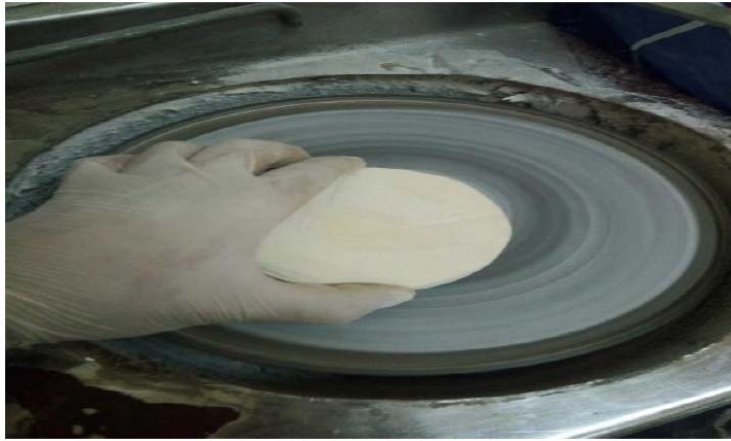
Figure S9: Manual polishing method using the EcoMet™ 30 polishing machine.
