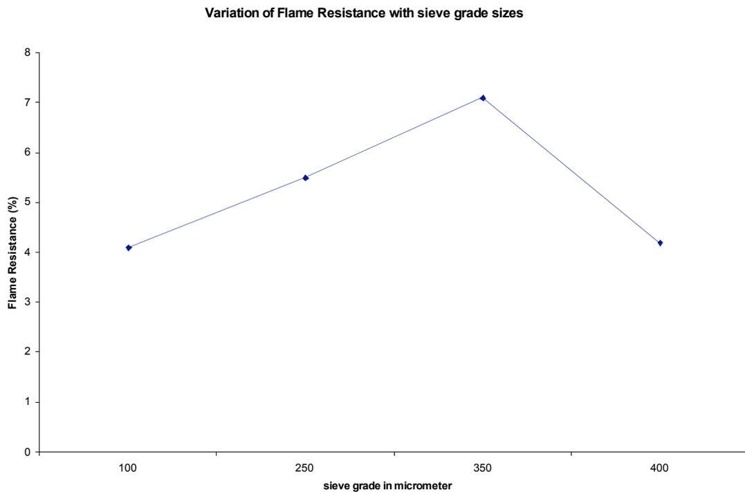
Figure 6: Variation of flame resistance with sieve grade sizes.
