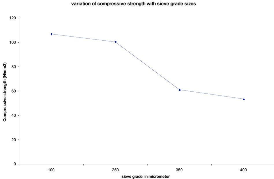
**Figure 4:** Variation of compressive strength with sieve grade size.
