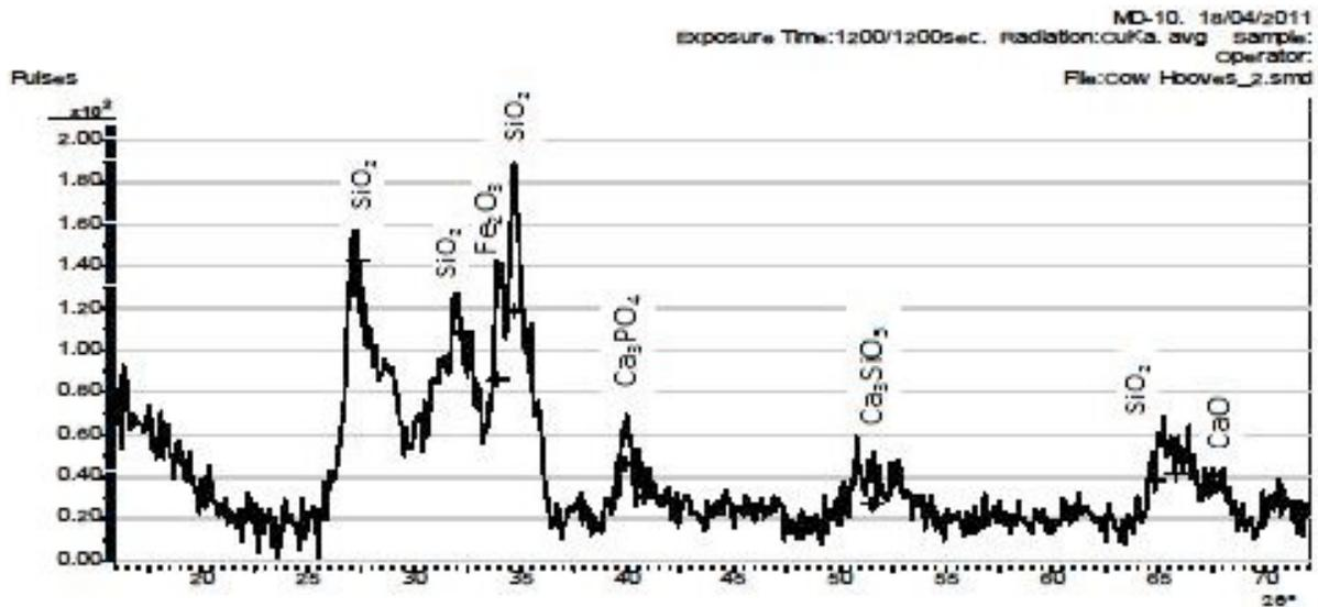
Figure 1: XRD spectrum for bagasse.
