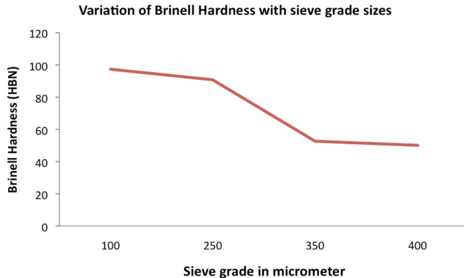
**Figure 3:** Variation of Brinellhardness with sieve grade sizes.
