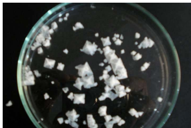
Figure 4: Irregular crystal formation result high magnesium content brine.
