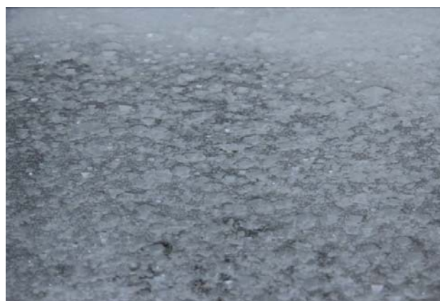
Figure 3: Well Shaped Pyramidal Crystals formation by Waste Brine.
