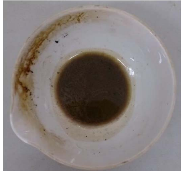
Figure 1: Sample of oilfield sludge.
