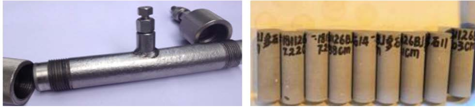
Figure 3: Sand-filled pipe for displacement (left) and artificial core (right).
