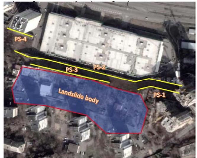
Figure 16: The orientation of retaining walls regarding the landslide body.
